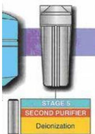
**Deionization** is a method used most often by laboratories to produce purified water on demand. All naturally-occurring water contains dissolved mineral salts. In solution, salts separate into positively-charged cations and negatively-charged anions. **Deionization** can reduce the amounts of these ions to very low levels through the process of ion exchange.
