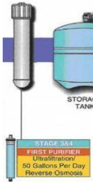
filtration system. The removal of up to 95 or 99.9% of undesirable water contaminants by forcing untreated water through a semi-permeable membrane. This process is called **Reverse Osmosis** because pressure forces the water to flow in the reverse direction to the direction of flow in natural osmosis. The multiple cleaning stages gives **Reverse Osmosis** its alternative name: **Ultrafiltration**.
